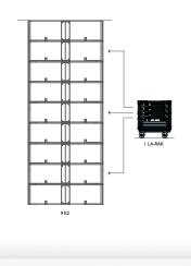
Presets: K2 line source: [K2 110] or [K2 70] or [K2 90] K1-SB, as an LF line source element : [K1SB\_X K2]
